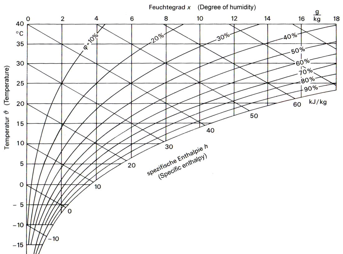
The relationship between the temperature, humidity and specific enthalpy of the moist air is summarised in the Mollier h/x diagram.
