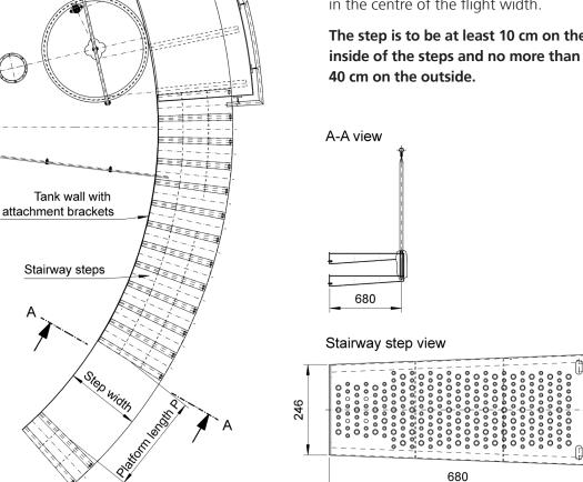
**Stairway** platforms A stairway platform is required at the beginning and end of each flight of stairs. In most cases, they are parts of storey ceilings or operator platforms.
